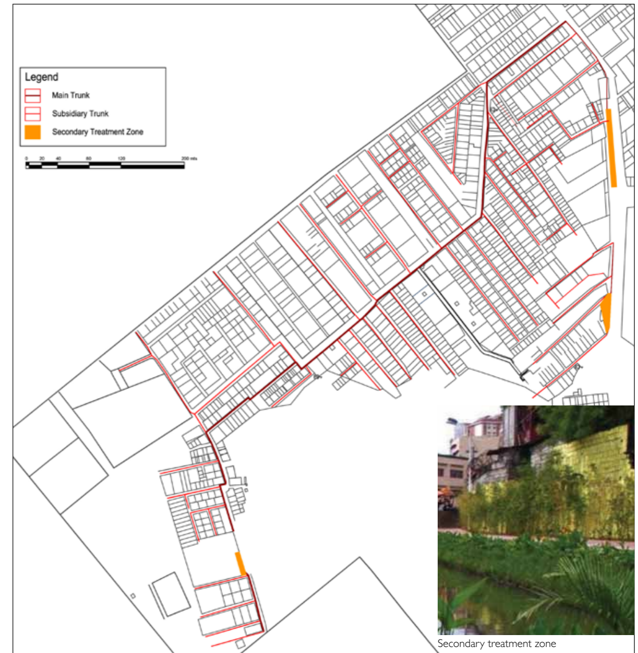
Drainage map of Phase 5 showing secondary treatment zones.
